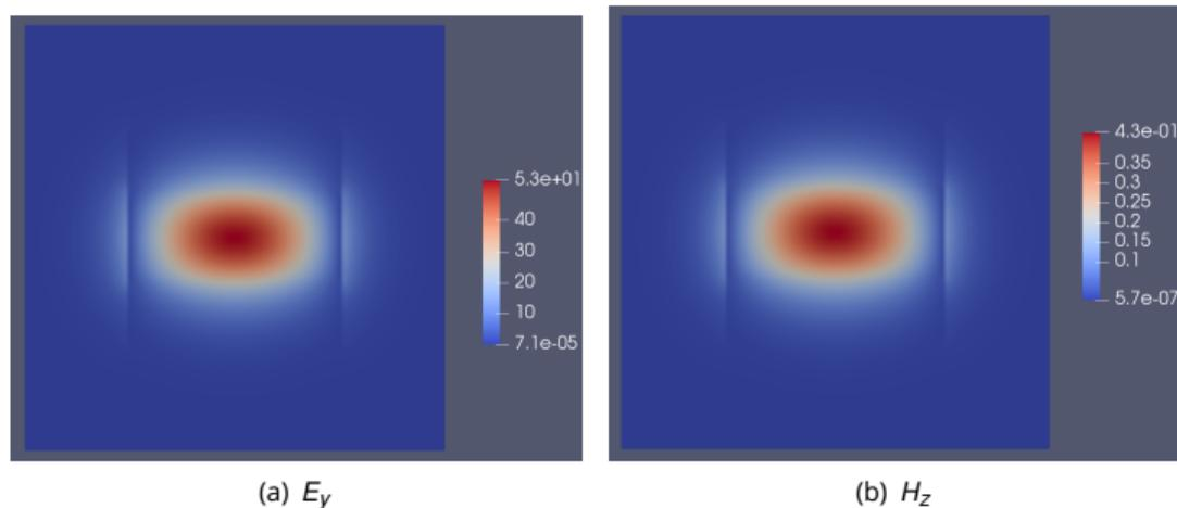
Figure:  $E_y$  and  $H_z$  of the calculated mode normalized such that the modal power is unity.
